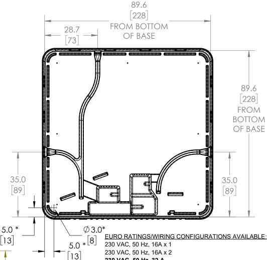
230 VAC, 50 Hz, 32 A 400 VAC, 50 Hz, 16 A x 3 (3 phase)
