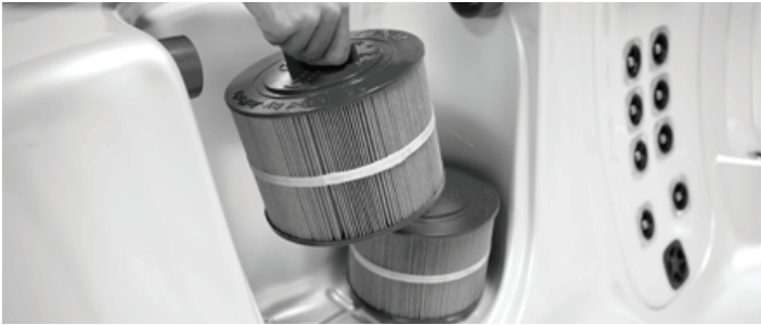
Step 4: Using a garden hose with a nozzle or other high-pressure device, clean cartridge(s). Work top to bottom on each pleat.
